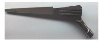
A sample of the femoral component of the hip prosthesis is shown in Figure 4.
