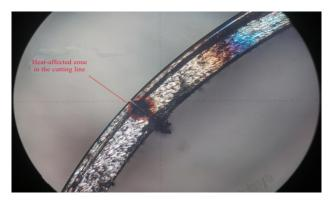
Fig.2. Heat affected zone inside the cut line at a slight increase of the radiation frequency
